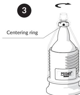
Fix the bottle by turning upper flask clockwise.
